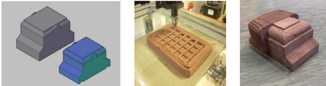
Figure 1. CAD-Model (left), 3D-printing of geopolymer fine mortar (middle) and demonstrator of the replicate sandstone (right)
